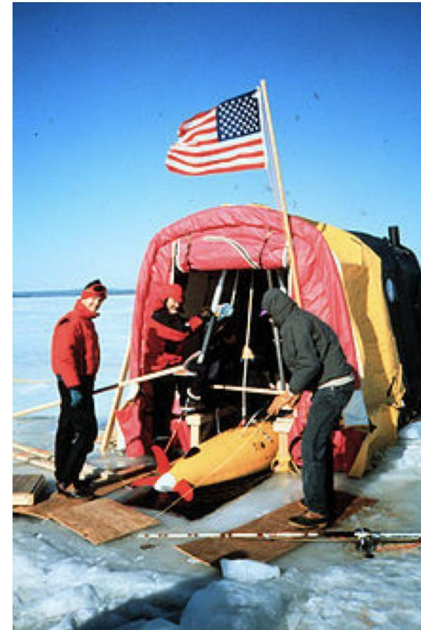
Figure 1: Arctic configuration of Odyssey II. Mission sensors are the scanning sonar at the nose, and the temperature and conductivity sensors located in the center of the vehicle.
