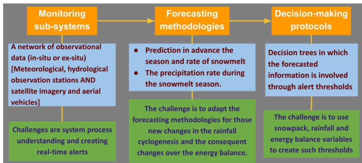
Figure 3: Highlights for an integrated flood warning system
